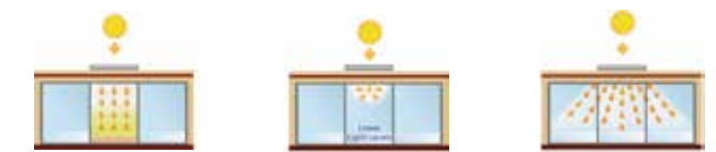
Differences in the light transmission and scatter with transparent, opal and prism glazing
