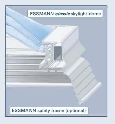
The skylight domes can be combined with all ESSMANN skylight base versions and are prepared for daily aeration and ventilation.
