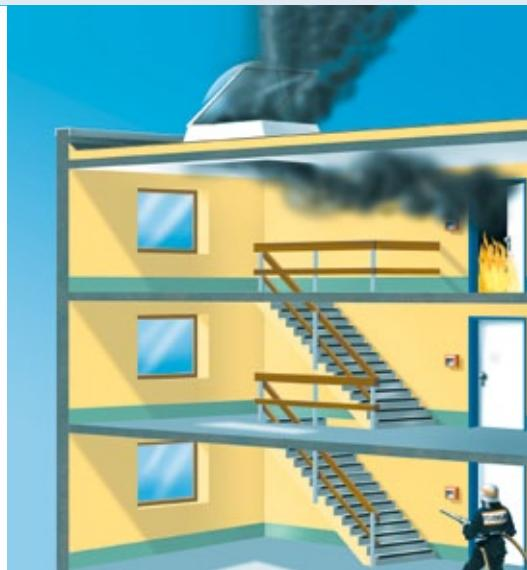
**ESSMANN egress hatch type M, for use as a smoke extraction (SE) system, regional building ordinance compliant, for staircases**
