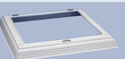
The **ESSMANN safety frame** for optional combination with the skylight domes of the classic range consists of a surrounding aluminium-reinforced and corner-welded hard PVC profile, which overlaps the roofing membrane that has been lifted up by 10cm around the base. The fastening hinges for the skylight dome are fully pre-installed on the safety frame at the factory.
