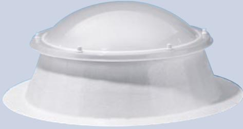
The **round ESSMANN skylight dome, fixed design** consists of high-quality, standard opal-coloured acrylic glazing (2 or 3-skinned), which is screwed directly onto a GRP base.
