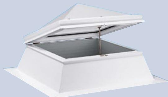
The **ESSMANN pyramid skylight dome** consists of high-quality, opal-coloured acrylic glazing inclined at approx. 30 degrees. It is provided with a hard PVC kerb frame and moulded drip edge and is ready for everyday ventilation. The acrylic skins are formed in one piece in the shape of a pyramid.
