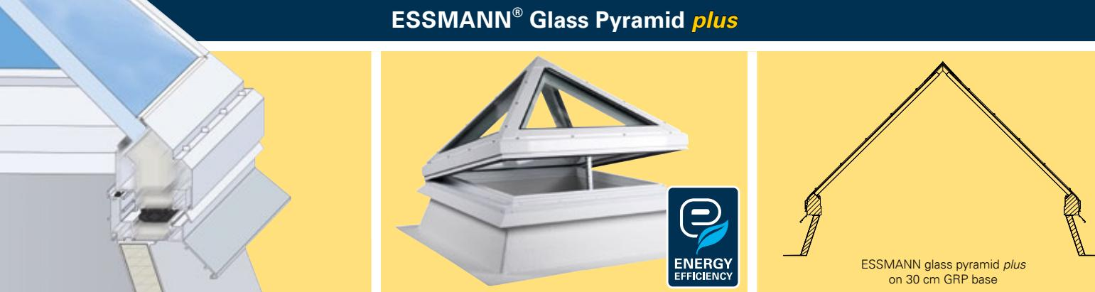
**ESSMANN glass pyramids *plus*** are completely pre-assembled as square pyramids (inclination angle 45°) and are fixed onto a heat insulated 30 cm high GRP base. The supporting structure consists of a high-quality aluminium profile system that is totally thermally separated. The aluminium profiles are powder coated in white (RAL 9016). The heat insulation glazing consists of double glazing as standard, the inner pane being made from compound safety glass (CSG).
