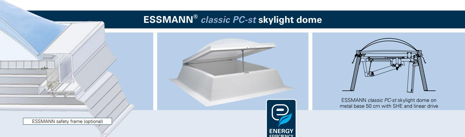
A transparent, flat polycarbonate panel is integrated into the kerb frame of the **ESSMANN classic PC-st skylight dome** (PC = polycarbonate / st = sheet top) together with one or two arched acrylic skins.
