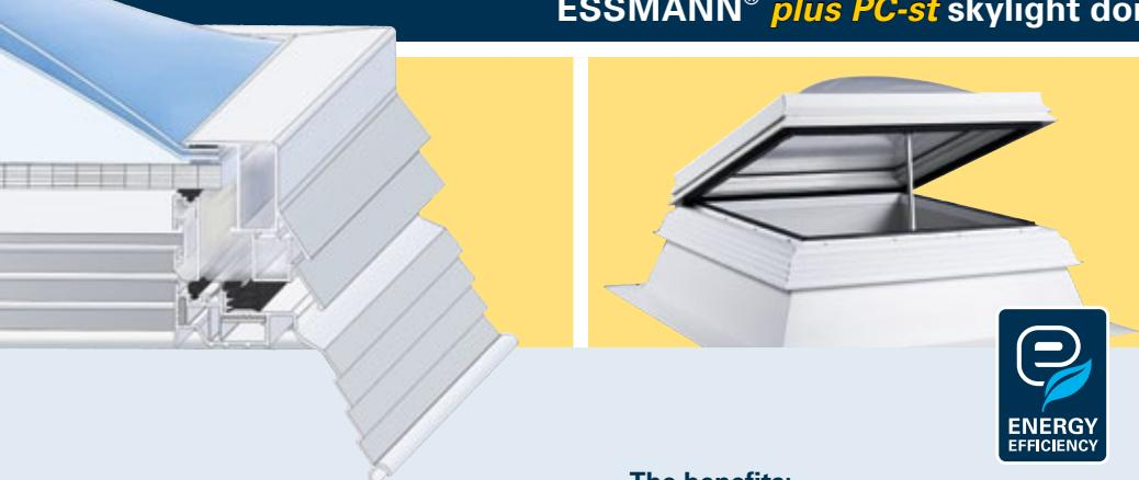
A polycarbonate web plate is integrated into the kerb frame of the **plus PC-st design** in addition to the acrylic skins. This produces even better u values and improves light transmission. Together with the system frame, the dome creates a visually homogenous unit - even in the area where the skylight base is joined. Two sealing levels at different heights and EPDM seals all around ensure excellent airtightness, thus significantly reducing the risk of heat loss.
